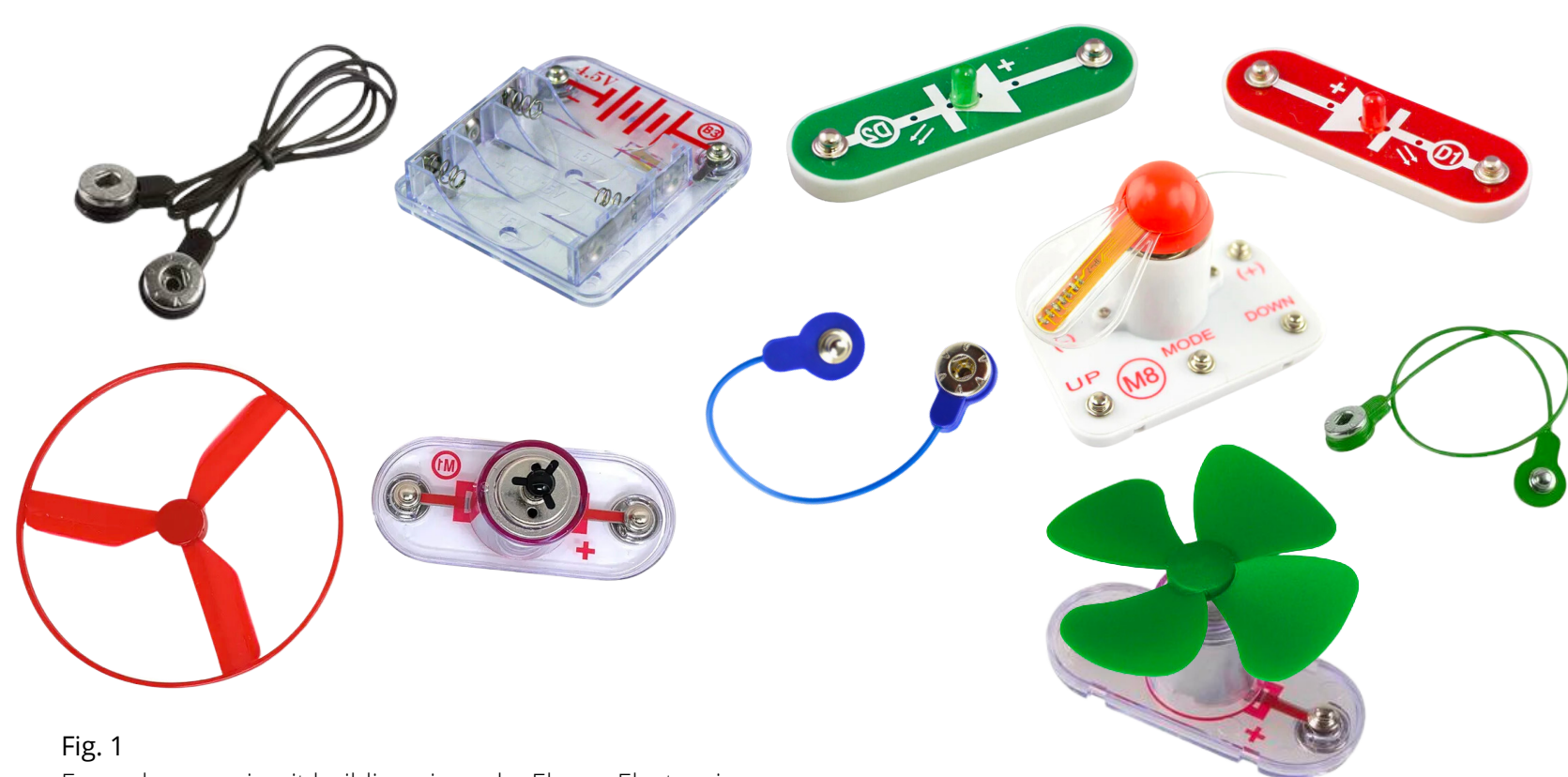
Fig. 1 Example snap circuit building pieces by Elenco Electronics, including LEDs, motors, fans, battery pack, and jump cables [9].
